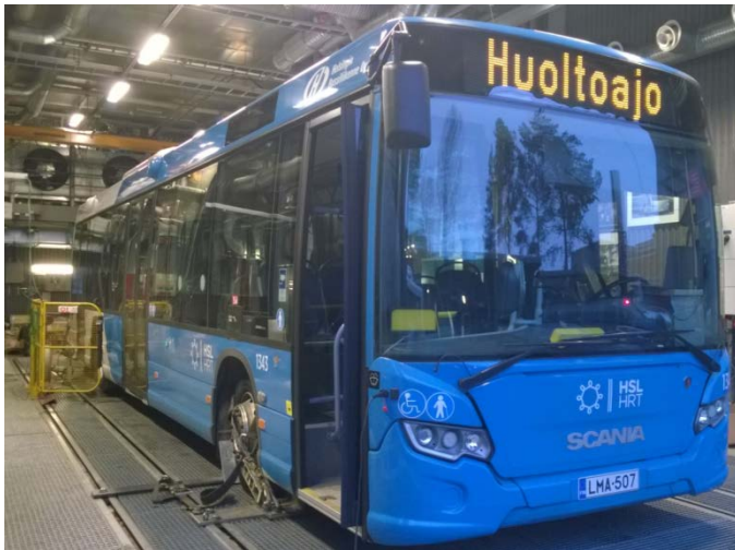
Fig. 2 One of the field test vehicles on VTT's heavy-duty chassis dynamometer
