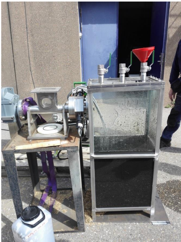
Figure 22: Picture of the gas tight tank
