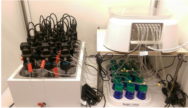
Figure 29: Equipment for BMP measurements
