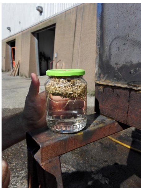
Figure 20: Straw after testing in a simple hydraulic press setup
