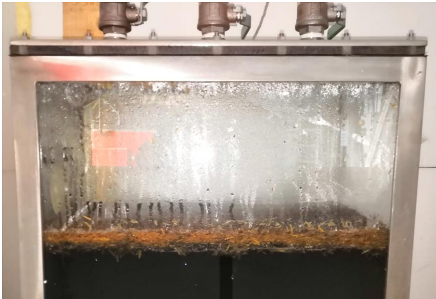
Figure 27 Top of the chamber after 34 days. Floating un-digested straw is on the surface
