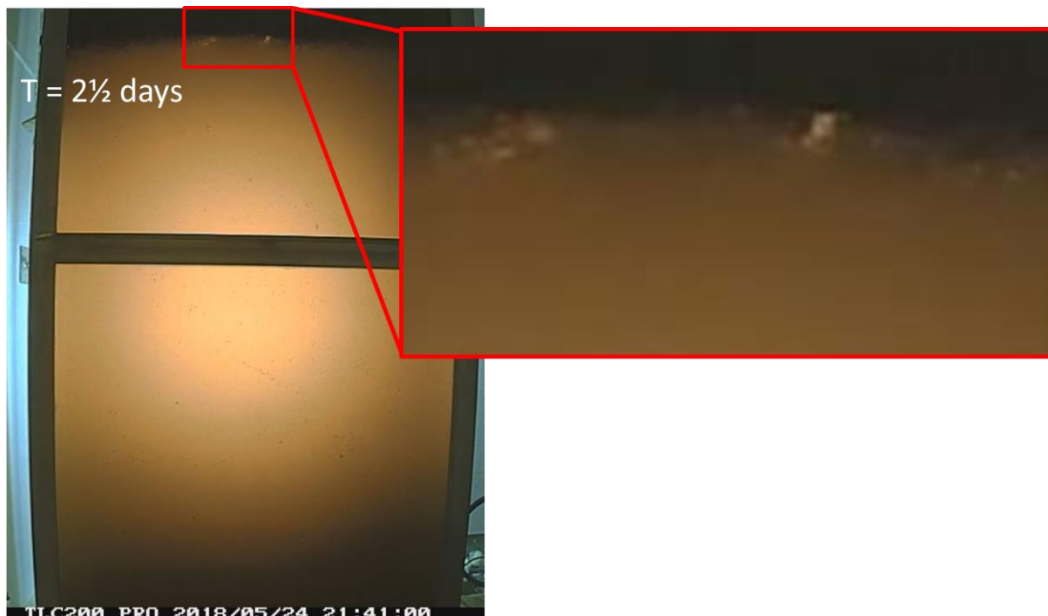
Figure 28 Gas bubbles under the floating layer after 2½ days
