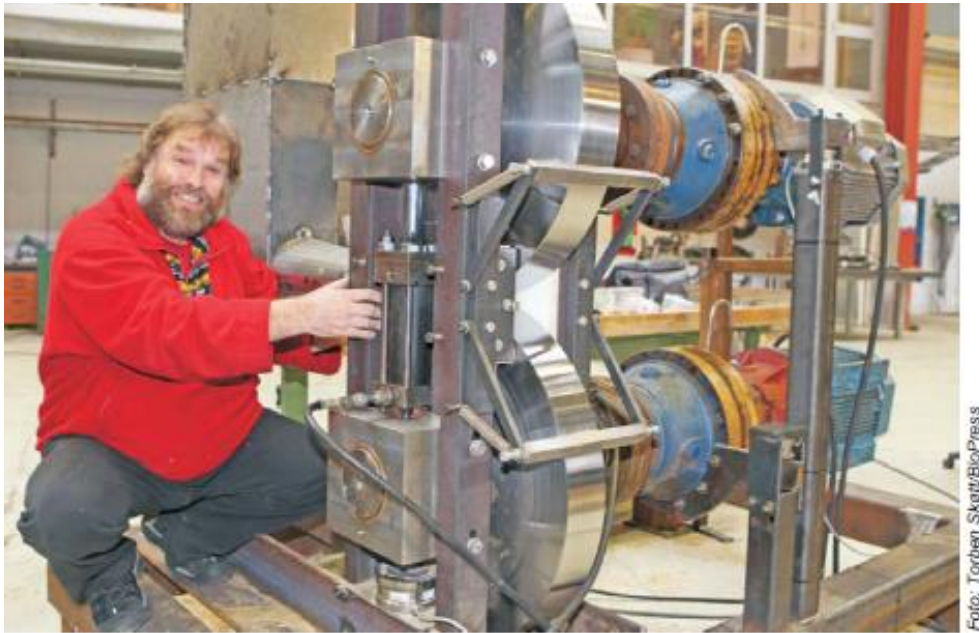
Figure 6: Custom built rolling mill for crushing of straw
