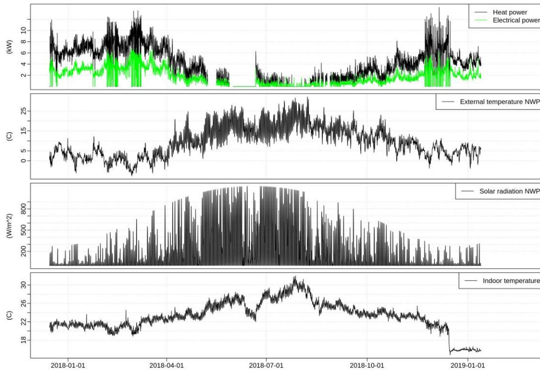
The activation periods in March and December 2018 can easily be seen. Further, it can be seen that the indoor temperature is around 22-23 C in the heating period, with some lower values during the activation periods.
