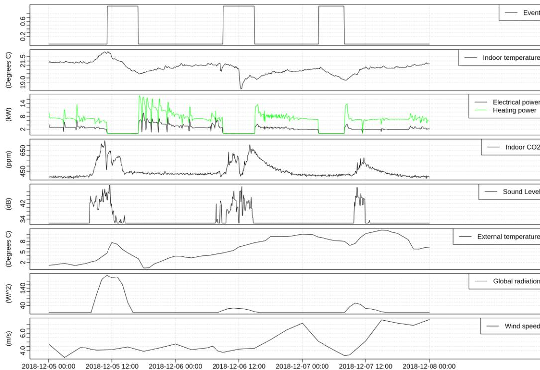
From which we find that a ventilation must have occurred, probably from window opening, since both the indoor temperature and the CO2 level drops very rapidly. From the experience gained when applying the models it is clear that this particular event does influence the results (not the forecasts themselves, but on the performance measures) it is chosen to remove it from the data set. In further studies more detailed analysis of the impact of such events should be carried out.
