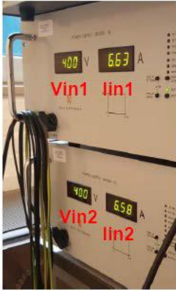
Figure 17 The low voltage side voltage balancing of the 110 V/220 V version converter.
