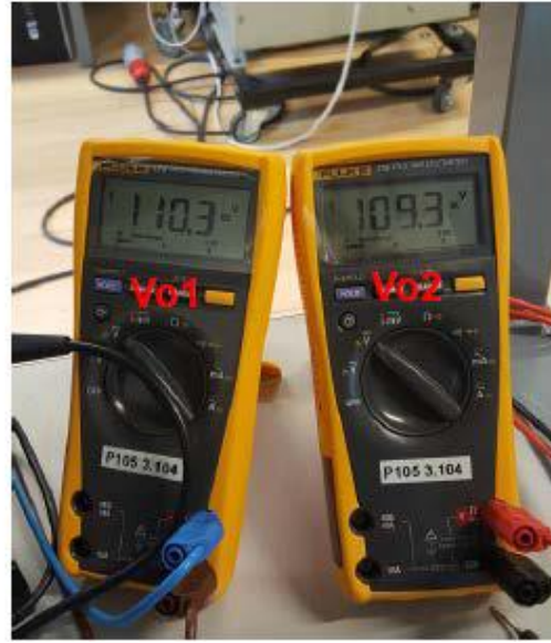
Figure 17 The low voltage side voltage balancing of the 110 V/220 V version converter.
