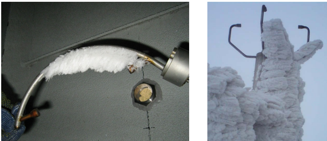
Figure 1: Ice build-up on non-heated spinner anemometer sonic sensor, left. On the right is shown ice build-up around a heated 2D sonic anemometer during the same event.
