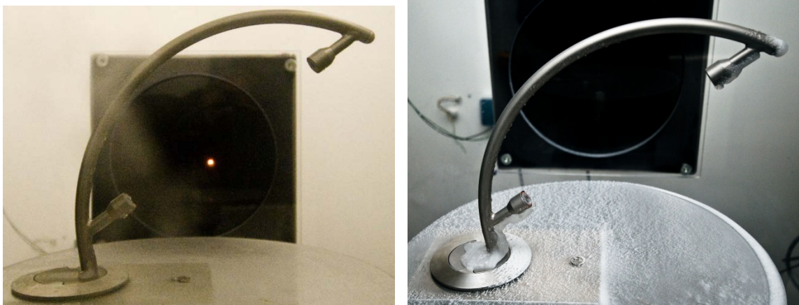
Figure 4 First test with heating applied during icing. Left, first visible ice on the lower sensor head after 10min. Right, ice build-up after 30min.
