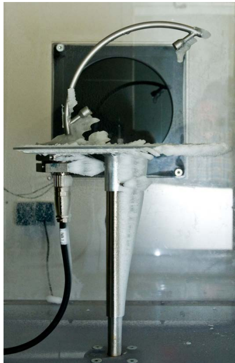
Figure 5 Melting of ice on the test setup after the second test.
