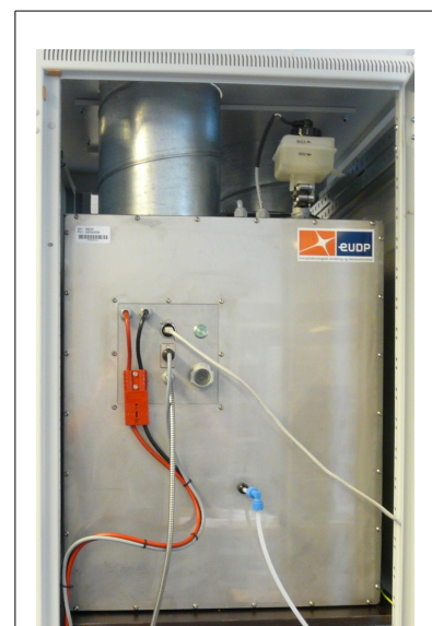
Illustration 14: DMFC in manifold
