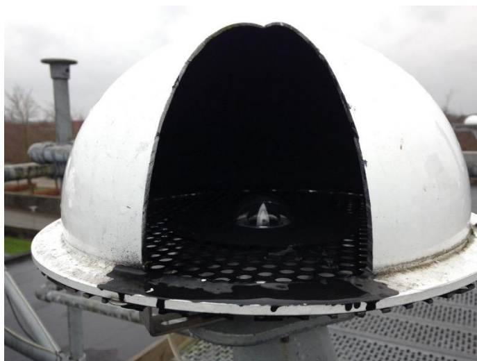
Figure 1.5: Experimental set-up with a pyranometer and a dome with 1/8 opening.
