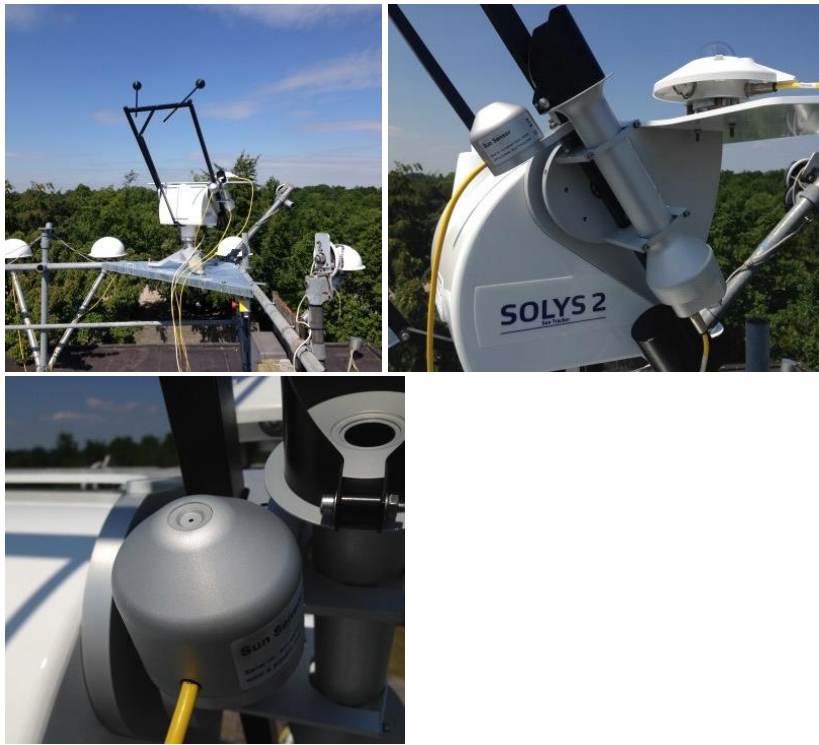
Figure 1.2: The SOLYS 2 tracker. On the top mounting plate, the pyranometer that measures the DfHI can be seen. On the left side of the tracker, the solar sensor and the pyrheliometer that measured the beam normal irradiance can be seen. Below the pyrheliometer, the solar sensor can be seen.
