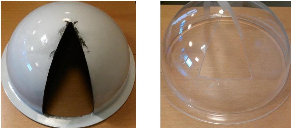
Figure 1.6: Left: dome with 1/8 opening area. Right: dome with 1/16 opening area.
