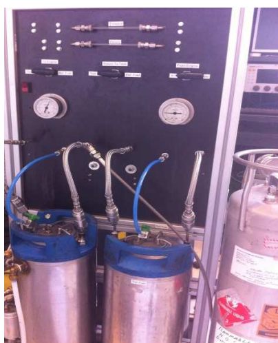
Figure 1 Fuel handling system
