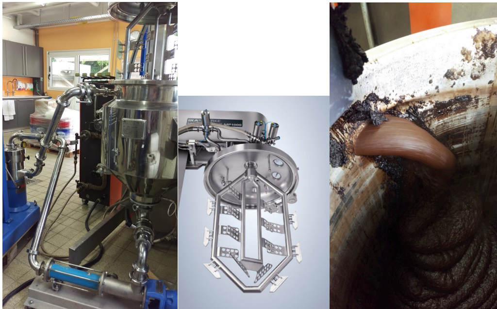
Figure 5: Slurry preparation using colloidal mill at IKA. To the left a slurry with a dry solid content of circa 20 wt % is shown.
