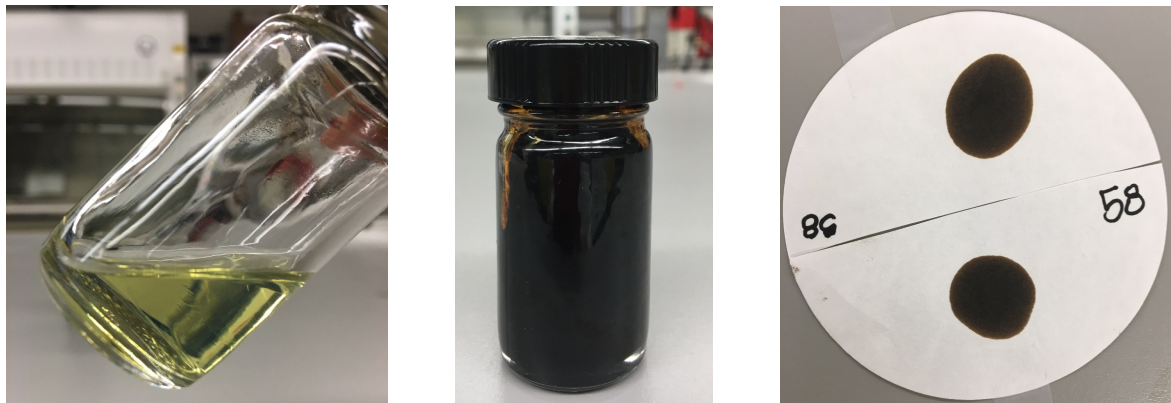
Figure 11: Left: 30 Renewable Diesel blend complying with the EN590 Ultra low sulphur standard. Right: Vial and Spot Test of the marine fuel blend (compatible).
