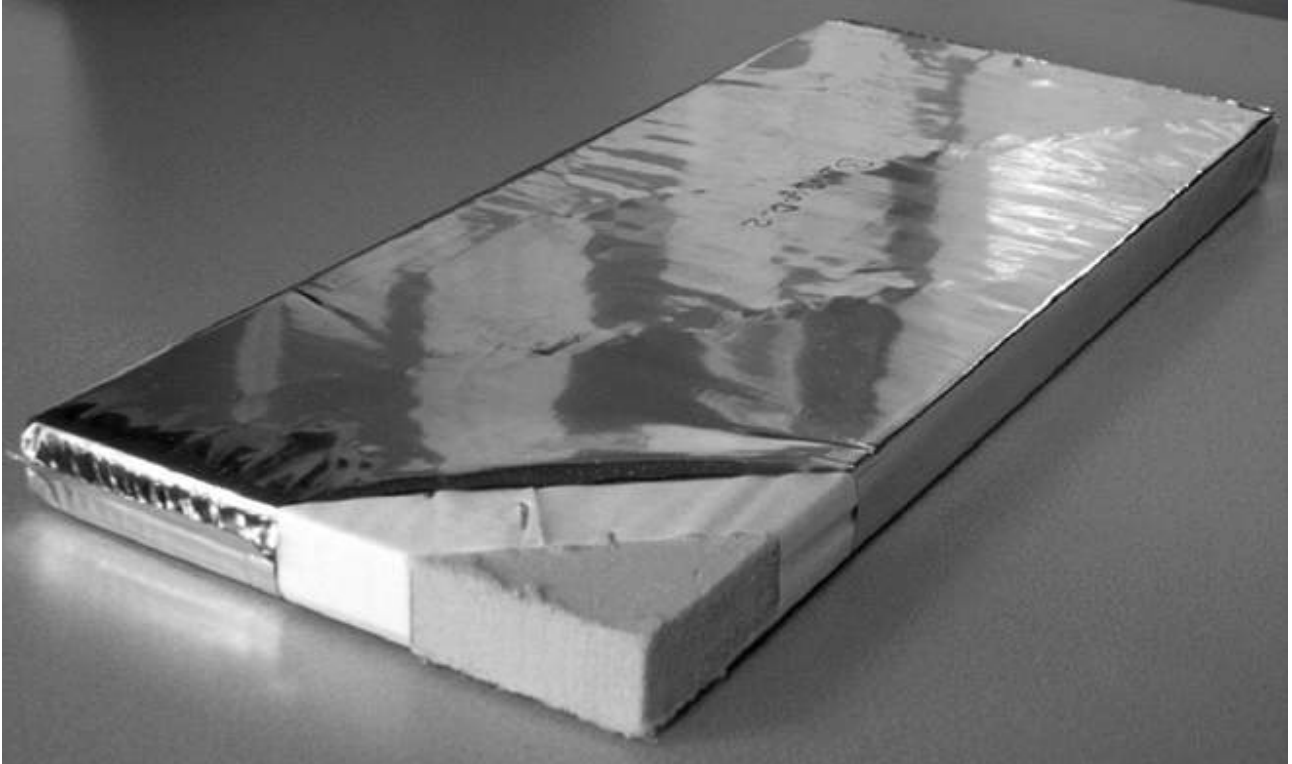
Figur 8: VIP insulation with the different layers exposed
