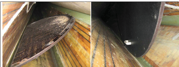
Figure 15: Loose blade lid inside the blade
