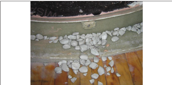
Figure 14: Separated glue rolling inside the blade
