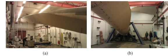
Figure 1 : SSP 34 m blade mounted on the test rig. (a) Root-to-tip view. (b) Tip-to-root view.
