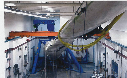
The 34 m wind turbine blade (top) is in the test facility at DTU's Wind Energy department's test facilities at Roskilde. A triaxial accelerometer (bottom) is mounted on the leading edge of a blade.
