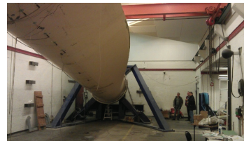
Figure 1. SSP34m blade mounted on the test rig
