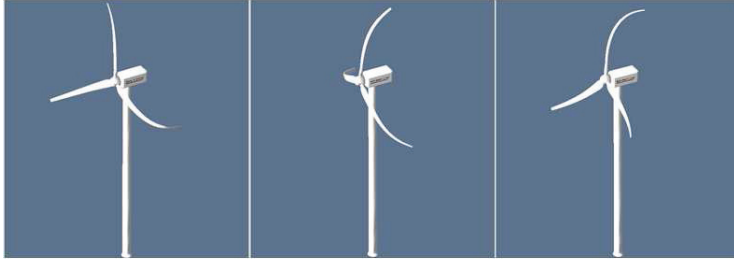
Figure 1: Components of the first flapwise mode
