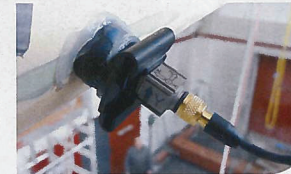
The 34 m wind turbine blade (top) is in the test facility at DTU's Wind Energy department's test facilities at Roskilde. A triaxial accelerometer (bottom) is mounted on the leading edge of a blade.
