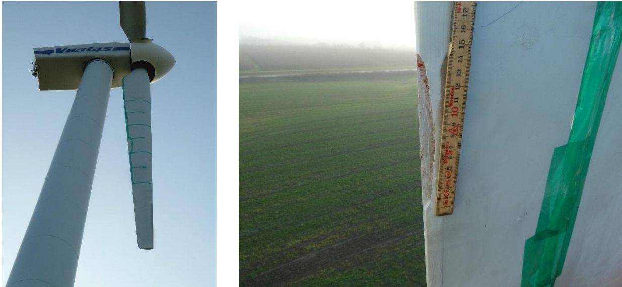
Figure 9. Left: Vestas V27 equipped with the blade SHM system. Right: the artificial 15cm trailing edge opening, which was successfully detected by the system.
