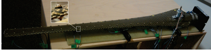
(a) Disposition of the bolts on the blade and blade support
