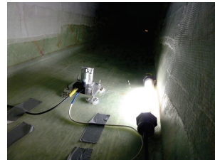
Figure 3. Mounting inside an SSP34m blade
