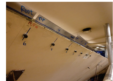
Figure 6. Bolts and metal plates used to change damage size in the second experiment.
