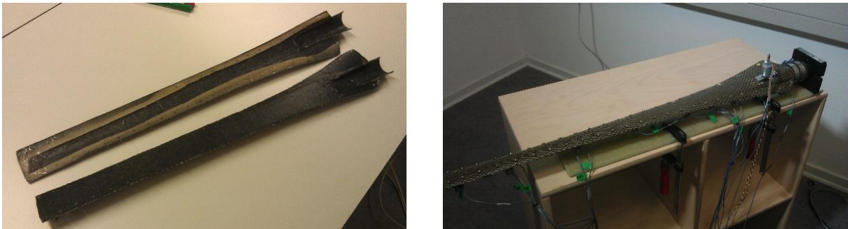
Figure 8. A 80cm blade from DTU Wind Racer project as a test object: left two halves; right – with mounted actuator and accelerometers
