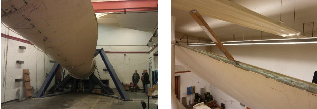
Figure 7. Left: SSP34m blade on a test rig. Right: an artificially introduced trailing edge crack.
