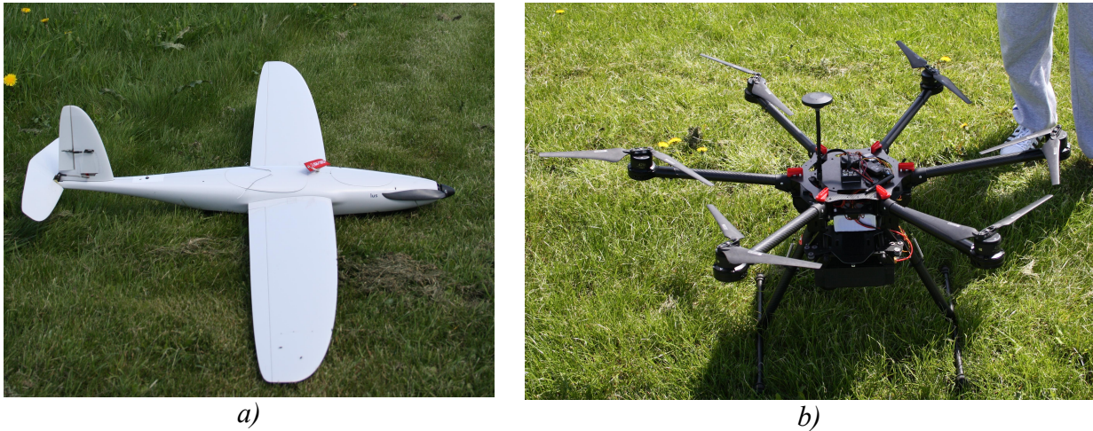
Figure 2. Drones used in the demo: a) fixed wing drone, Cumulus from Sky-Watch, b) hexacopter
