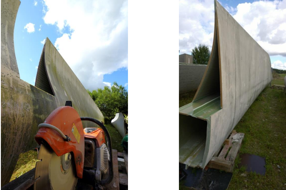
Figure 14. SSP34 blade with leading and trailing edge sections removed prior to and following spar sectioning at R15m - ready for transport to DTU MEK for substructure testing
