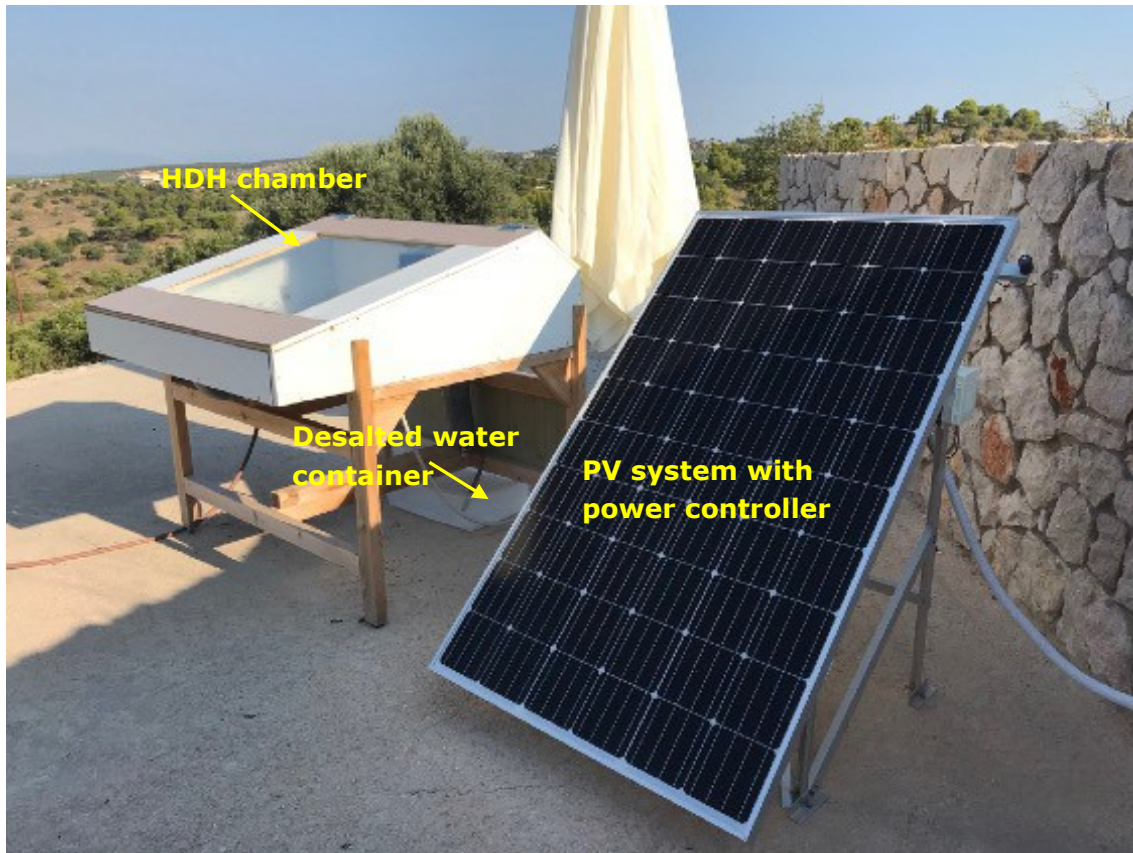
Figure 7. Fully functional PV-TE desalination system.
