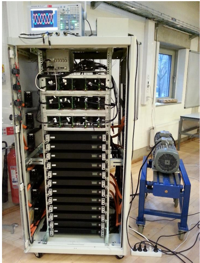
Figure 4: Multilevel converter with integrated battery modules. Top: System diagram. Bottom: Laboratory system.
