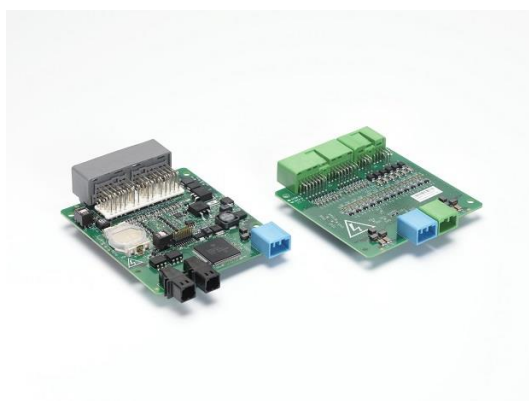
Figure 8: Automotive grade n-BMS platform developed by Lithium Balance
