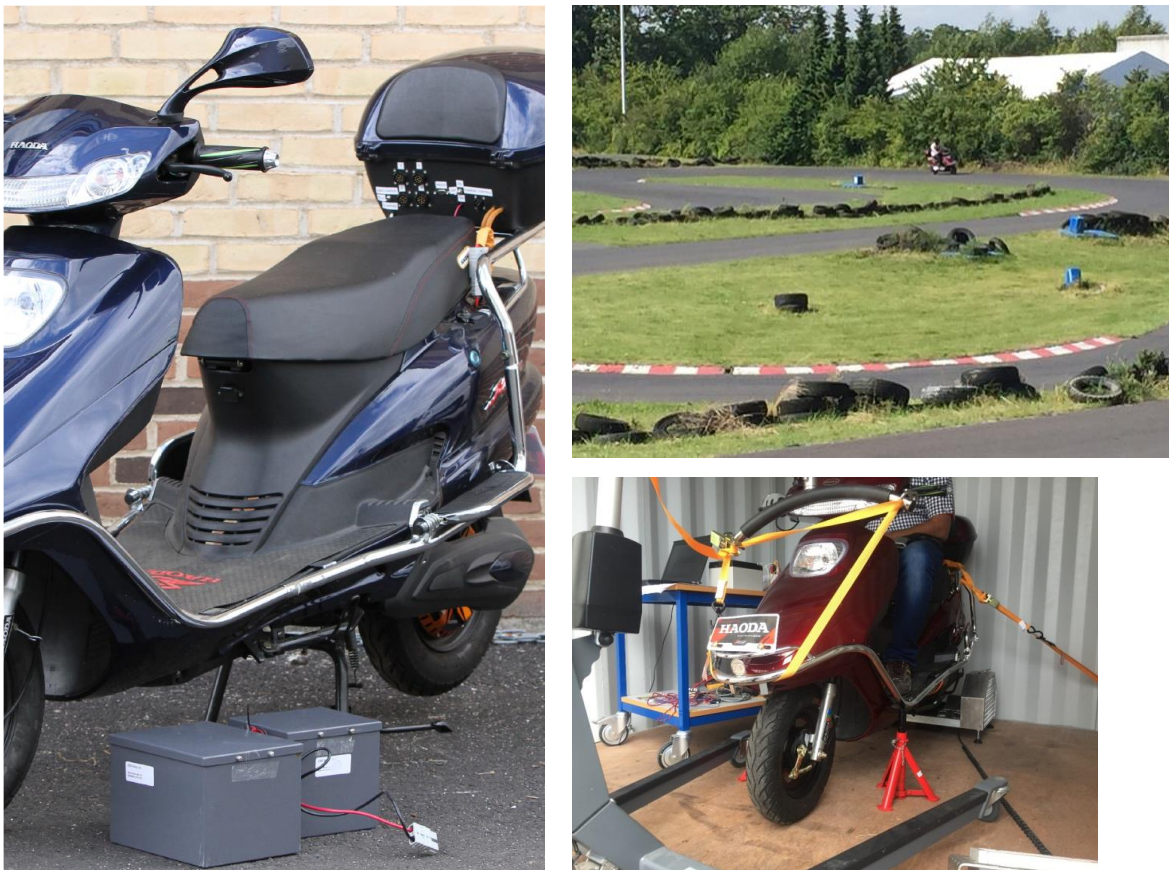
Figure 1: Electric-scooter used for demonstration of Li-S batteries.
