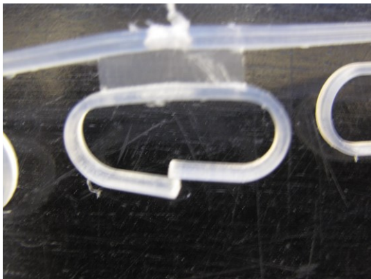
Figure 2.3.f. Fracture of injection moulded Hyflon. The fracture may be avoided by adjustment of the mould design.
