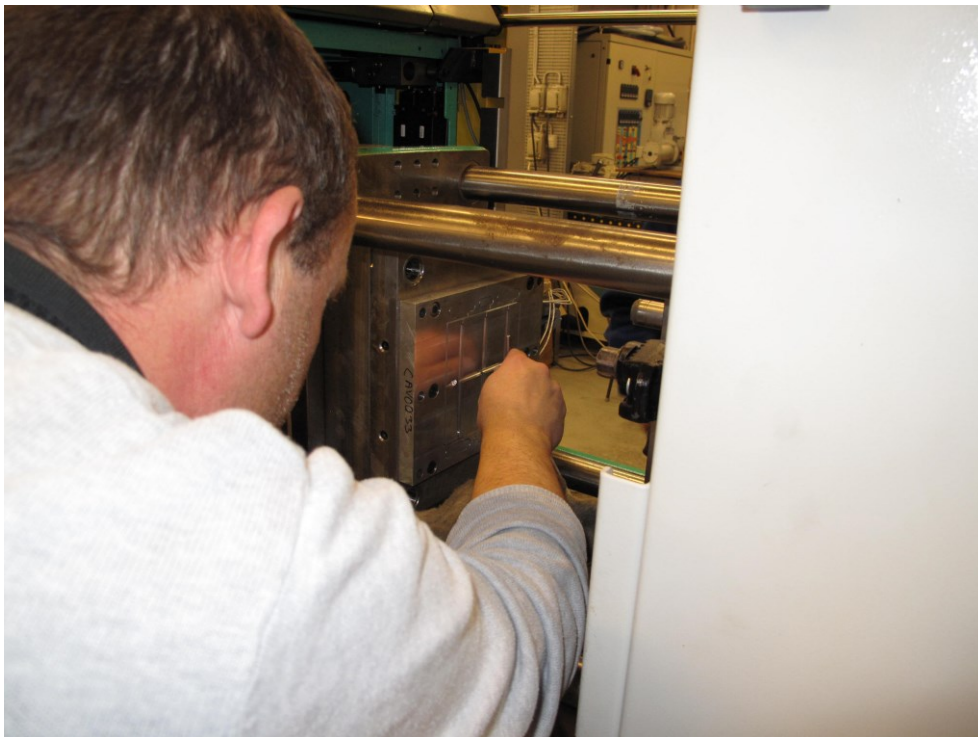
Figure 2.3.c. Injection moulding of fuel cell sealings. The mould is developed by IRD. A setup for processing of high temperature polymers has been developed.
