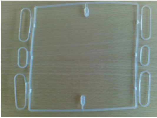
Figure 2.3.d. Injection moulded sealing of Hyflon MFA F1530. Process cycle = 5 min.
