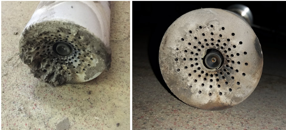
Figure 9. Left: Camera front with "shower head" from position in the right side of the boiler after few days of operation. Right: Camera front with "shower head" from position at the end of the boiler after weeks of operation.
