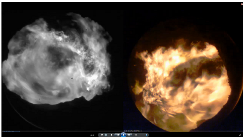
Figure 11. Simultaneous snapshots of video streams from cameras in side walls. Left: NIR camera in right side. Fuel travels from left to right. Right: RGB camera in the left side. Fuel travels from right to left.
