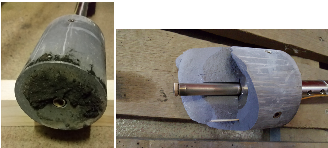
Figure 10. Left: Special designed ceramic dummy installed instead of "shower head" of the side wall camera. Right: Damaged ceramic dummy.
