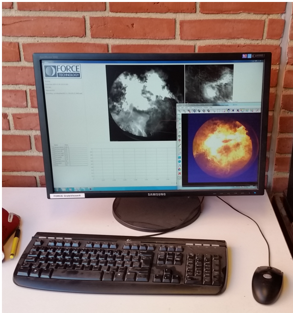
Figure 8. GrateVision® user interface on FORCE Technology PC in the control room. The B/W GrateVision window is using NIR camera in the right boiler wall. The colour picture is livestream from RGB camera at the end of the boiler.
