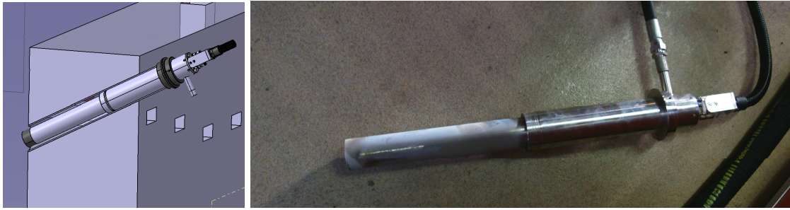
Figure 5. Left: Drawing of camera housing placed in guide tube in boiler wall. Right: Picture of camera housing.
