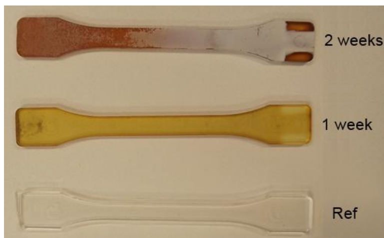
Figure 19. After being exposed to a combination of a highly aggressive chemical environment and elevated temperature for two weeks, this polymer test sample shows significant weight-loss and change in visual appearance. For this reasons this polymer is found to be unsuitable for cell frame material.
