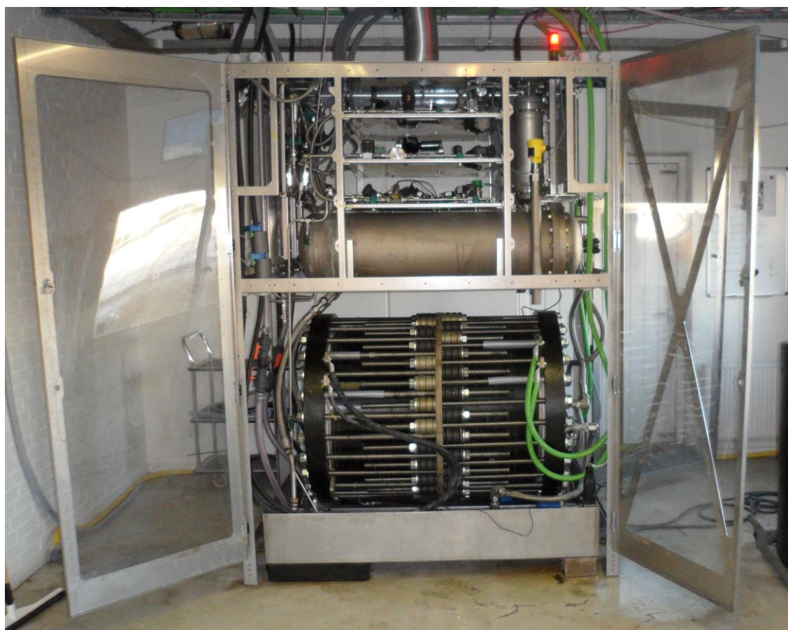
Figure 2. Prototype of the HyProvide 250 electrolyser unit being tested in GreenHydrogen's laboratory.
