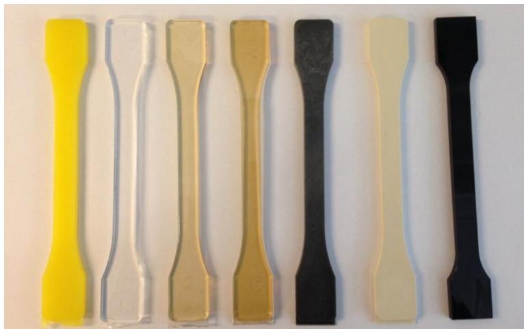
Figure 18. Tensile test bars made from different polymer types are tested in order to find the most suited polymer material for the cell frame. Mechanical strength, thermal and chemical stability of the polymer materials is investigated.
