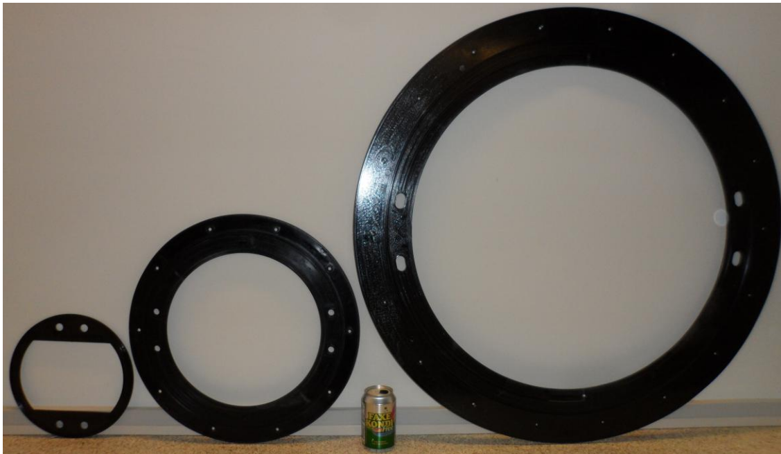
Figure 16. These cell frames are used for construction of the GreenHydrogen stacks. Left: cell frame developed prior to the HyProvide project (270cm 2 active area). Center: cell frame for intermediate stack (705cm 2 active area). Right: cell frame for target stack size for the HyProvide project (3000cm 2 active area).
