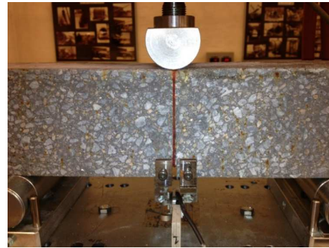
Three point bending tests on sawn out beams for determination of K factors
