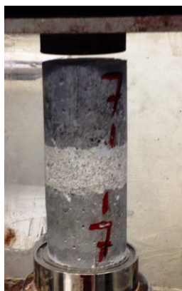
Cylindrical specimens with epoxy joints before and after testing
