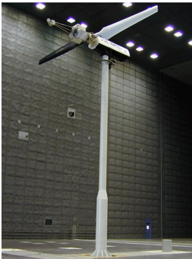
Figure 1 The NREL UAE Phase VI experiment in the NASA Ames 24.4 m x 36.6 m wind tunnel.
