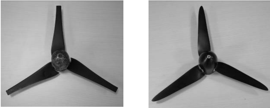
Figure 19: Photos of both rotors designed with the BE/M (left) and BE/LL (right) theories
