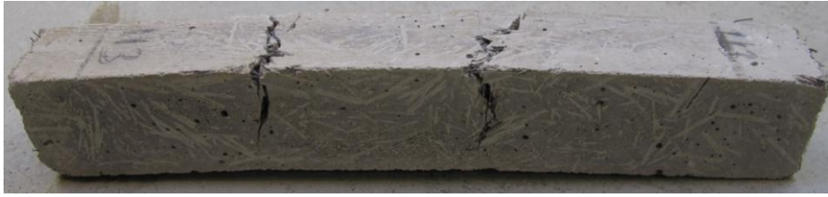
Figure 2, typical rectangular bar test specimen used to determine bending strength
