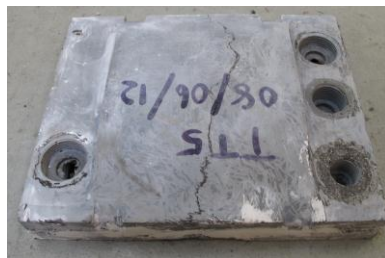
Figure 18. End plate following bending test
