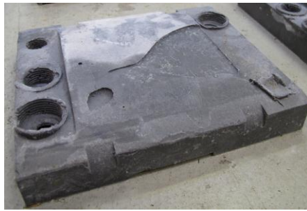
Figure 17. Endplate with defects around thread and large pores on the top surface
