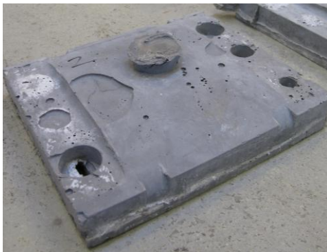
Figure 15. Endplate with defects from residual air bobses
