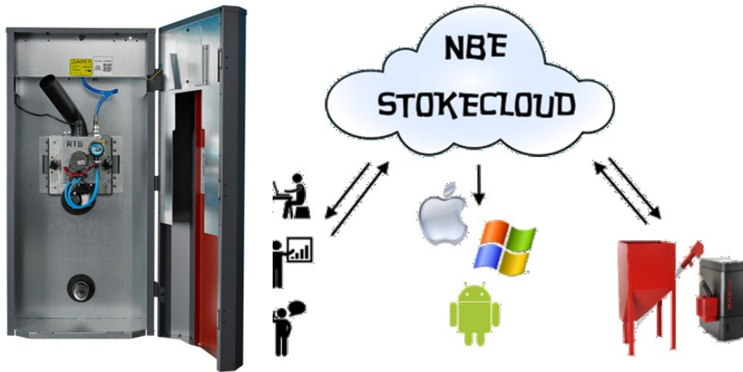
Figure 6 Principle behind NBEs StokerCloud
