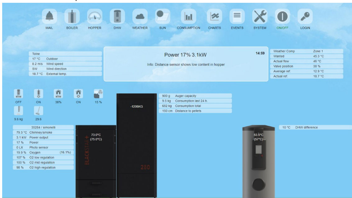
Figure 7 User interface for NBE boiler system
