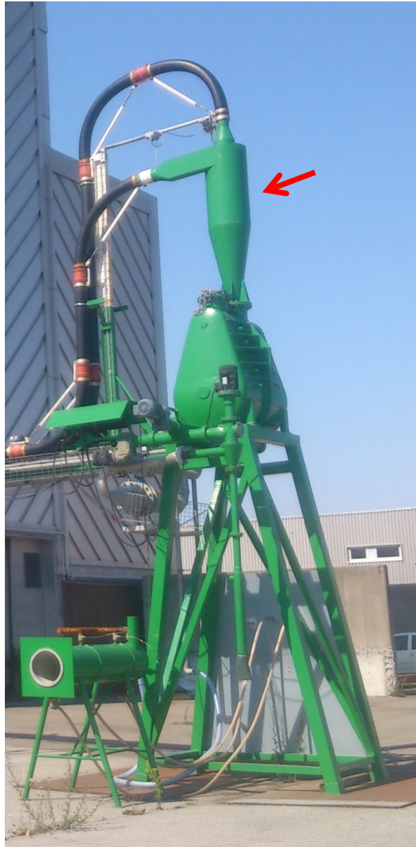
Figure 30 Picture of the cyclone on top of the dosing bin
