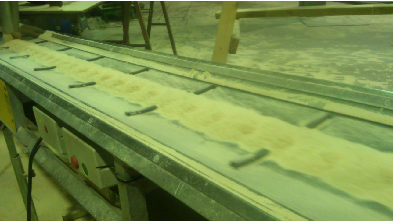
Figure 67 "Packs" of powders at the outlet of the injection unit
