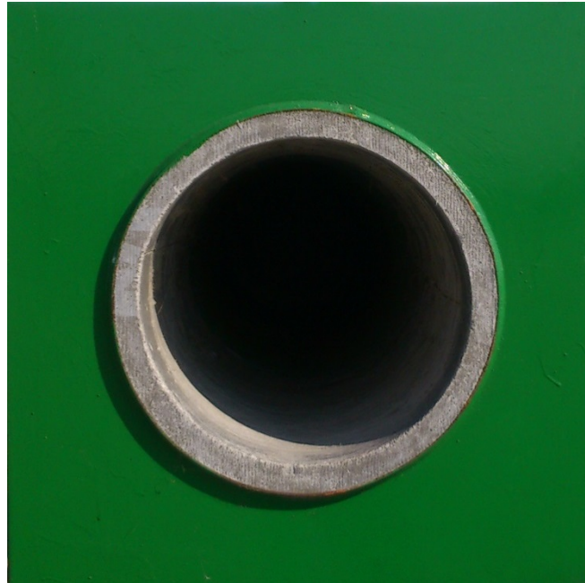
Figure 43 Picture of the gasifier (outlet) and its concrete inner layer
