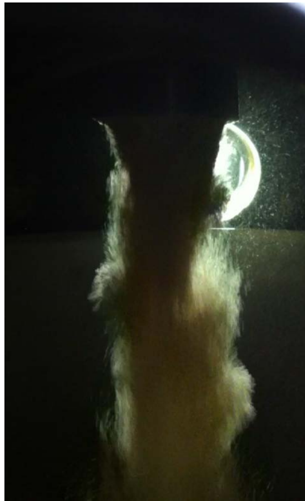
Figure 81 Pictures of wood powder injection into atmospheric and pressurized vessels
