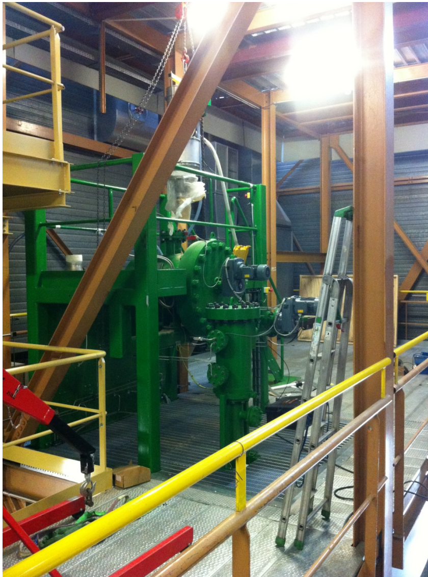
Figure 70 Picture of the first floor of the facility with the dosing bin and the injection cone vessels
