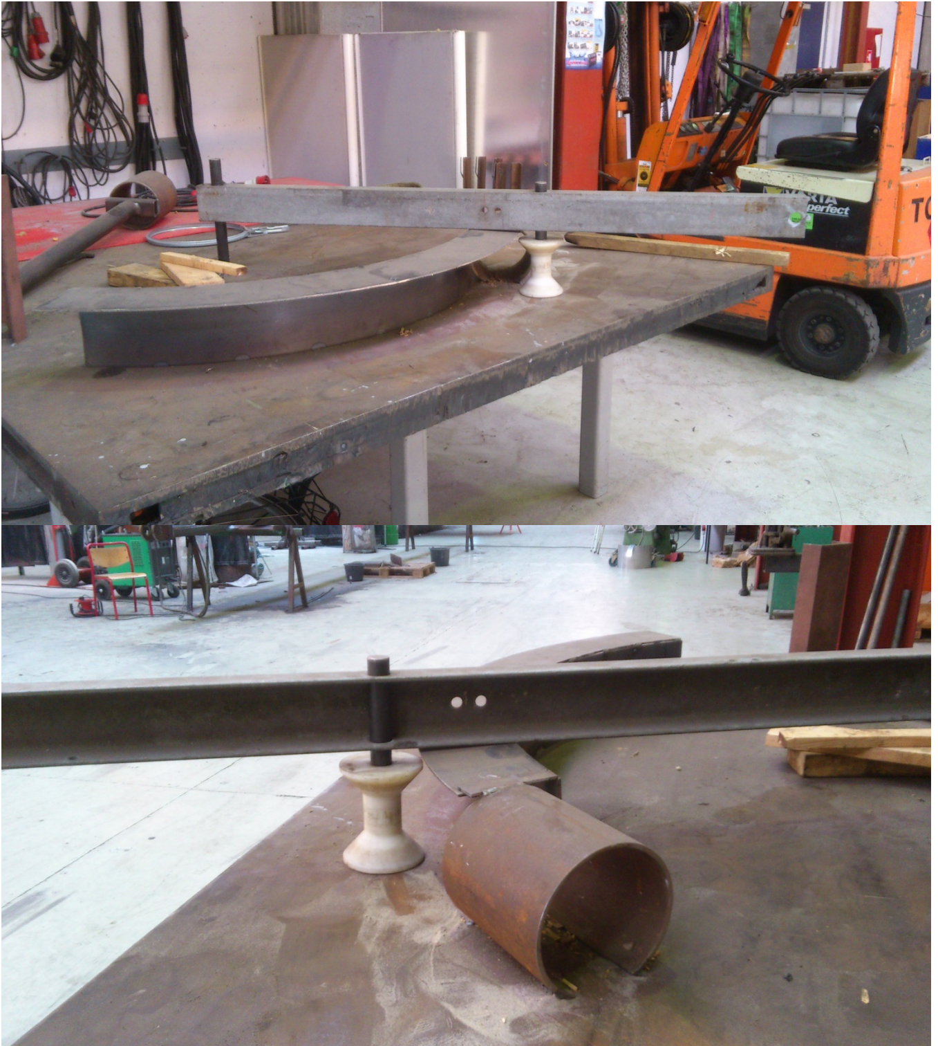
Figure 31 Pictures of the bending tool for PVC pipes
