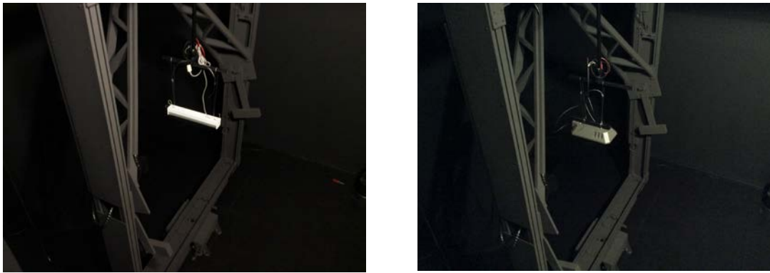
Figure 5 The four artefacts in IC2017 as mounted in the near-field goniophotometer at DTU Fotonik, top left: ART-1, top right: ART-2, bottom left: ART-3, bottom right: ART-4.
