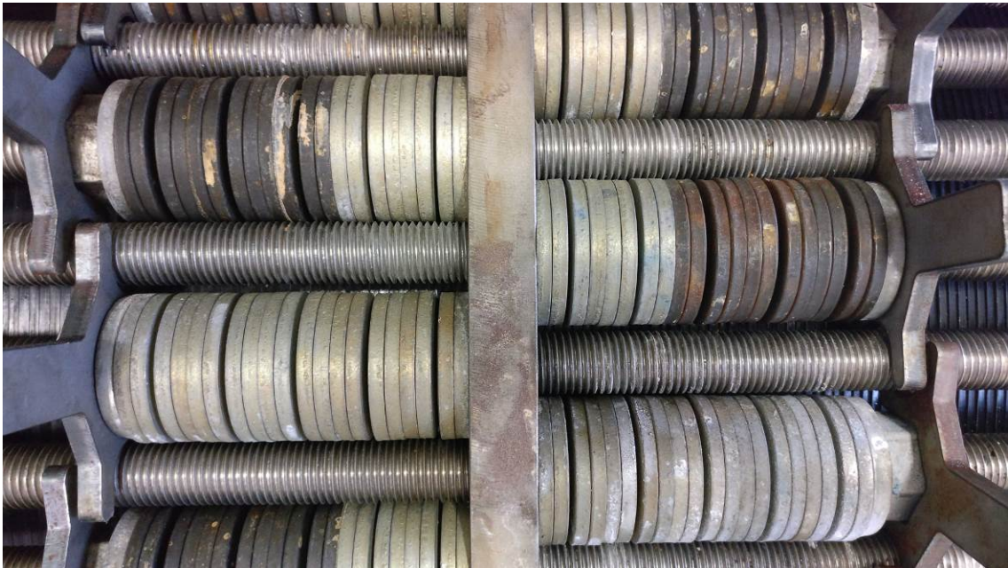
Figure 6 A view of the springs on the stack. It should be noted that all parts seen are some grade of carbon steel, The black disc springs are phosphorized spring steel and the white disc springs are Zink galvanized with chromate treatment. As seen on the picture, a small amount of surface rust is present on some of the phosphated springs. For The chromated springs the electrolyte is very corrosive to the zinc, so for most springs discolored white areas can be seen, where the spring have been in contact with KOH. It should be noted though, that this discoloration is of very little significance to the integrity of the spring. As the spring will only begin to corrode once a significant portion of zinc has been completely corroded away. And even with the rugged treatment in the laboratory, none of the chromated disc springs show sign of corrosion in the steel beneath the plating.
