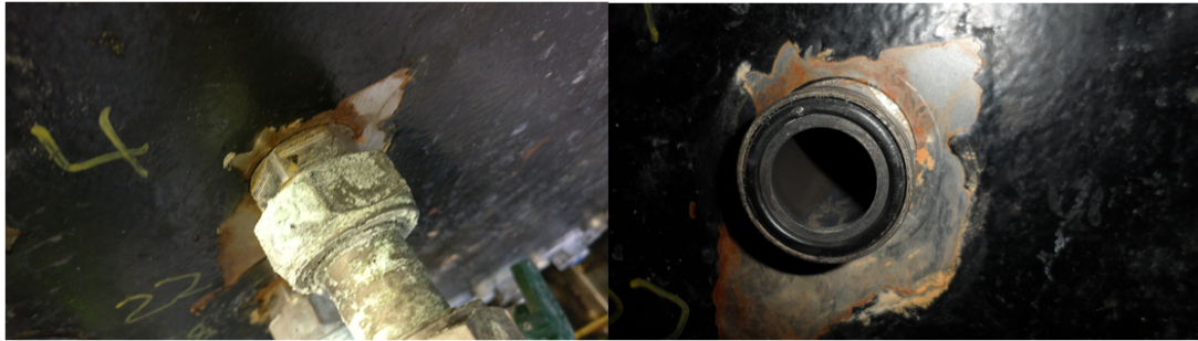
Figure 3 – Hydrogen outlet at the end flange. The white crystals in the picture are KOH crystals. Nearest the flange is seen an inserted Monel body. With the flange made from carbon steel. It is seen that some surface rust is present on the flange where the painting have been scraped off. The monel body is very resistant to corrosion, and still shine if wiped clean. One thing that should be noted is the slightly green color of the swivel and gland. These parts have been coated with electroless nickel where the slightly green color indicates some nickel is present in the KOH crystals. Meaning some nickel from the plating has been dissolved. There is however no indication that this corroded nickel is of a significant magnitude, as the electrolyte does not appear to become green in the same manner. (or take on any other strong color for that matter.) There is a slight blackening of the inside surface, and some sludge seen in the fitting. The subtle red tinge on the on the Picture on the Monel part is not rust from the Monel, as there is no Iron in the Monel alloy
