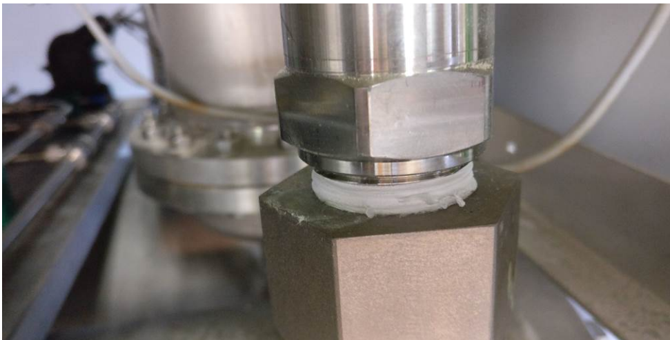
Figure 5 – Connection between the level sensor and the level sensor tube. No outside visuals indicate any corrosion. However, this connection is the only one in the machine with a threaded seal connection, that is also coated with Ni, and further, it is also a 1" connection, making this seal one of the most problematic in the machine. Making the connection tight have proven to give some difficulty. However, the good news for this connection is that it is neither exposed directly to electrolyte or temperature. So corrosion in the thread is very slow.
