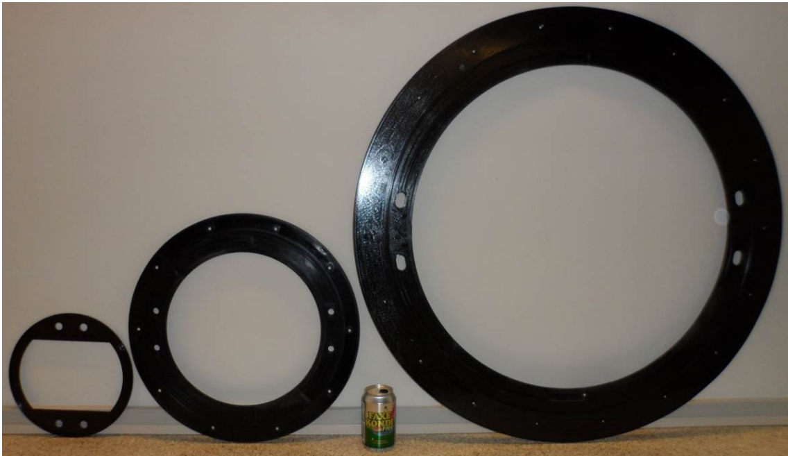
Figure 10 - Cell frame sizes of the different stack generations, 2, 12 and 60 Nm 3 /h
