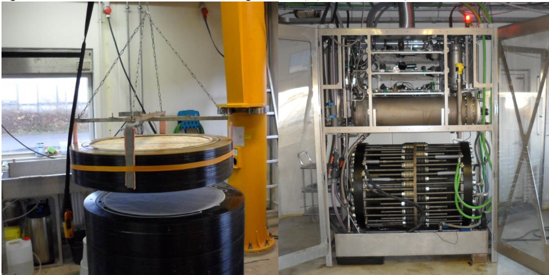
Figure 11 – Construction of the Cell Stack. And the full prototype in operation (The red light on the top of the machine indicates the system is powered and pressurized)
