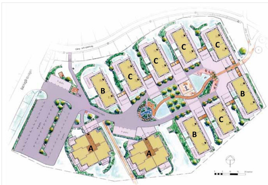
Figure 56. Principal site plan of the Söndrums Kyrkby multi-family and pair passive house ground site. Building types are: (A) Multi-family houses, (B) Pair-houses with a two-room and a four-room apartment, and (C) Pair-houses with two three-room apartments. Source: [3].
