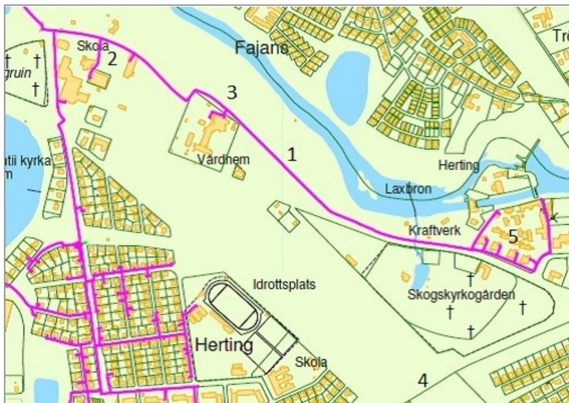
Figure 51. Overview of heat distribution pipe line to Hertings gård from Falkenberg city district heating network. Source: [16].
