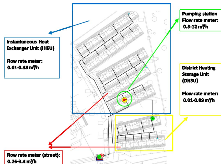
Figure 3 Sketch of the DH network with the location of the meters.
