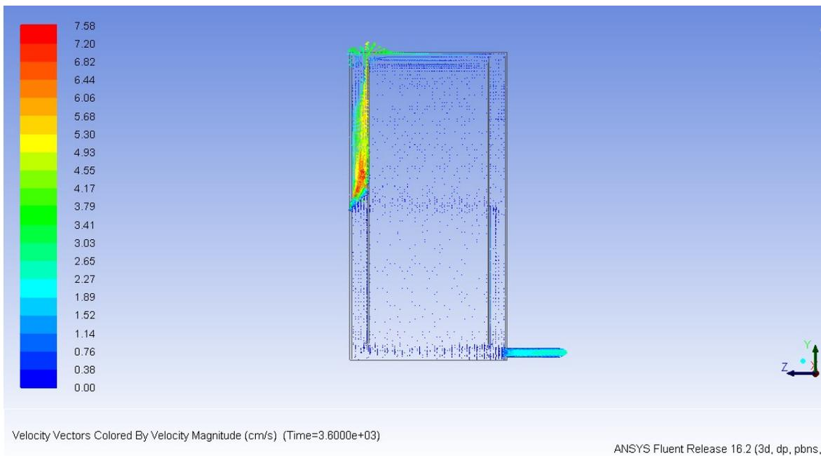
Figure 3. Water velocities in the heat storage during charge.
