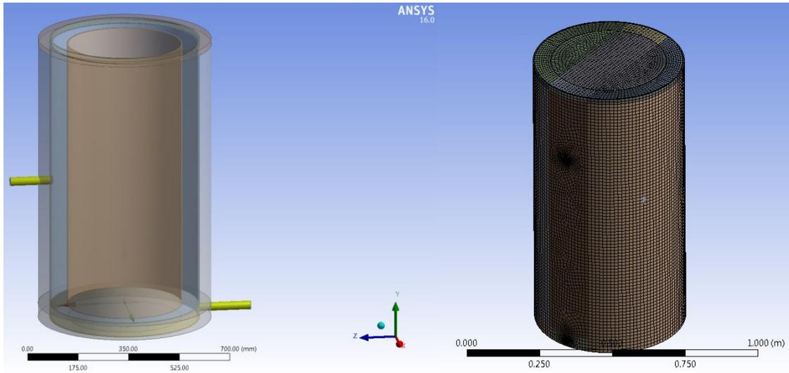
Figure 2. Mesh of tank in tank heat storage.
