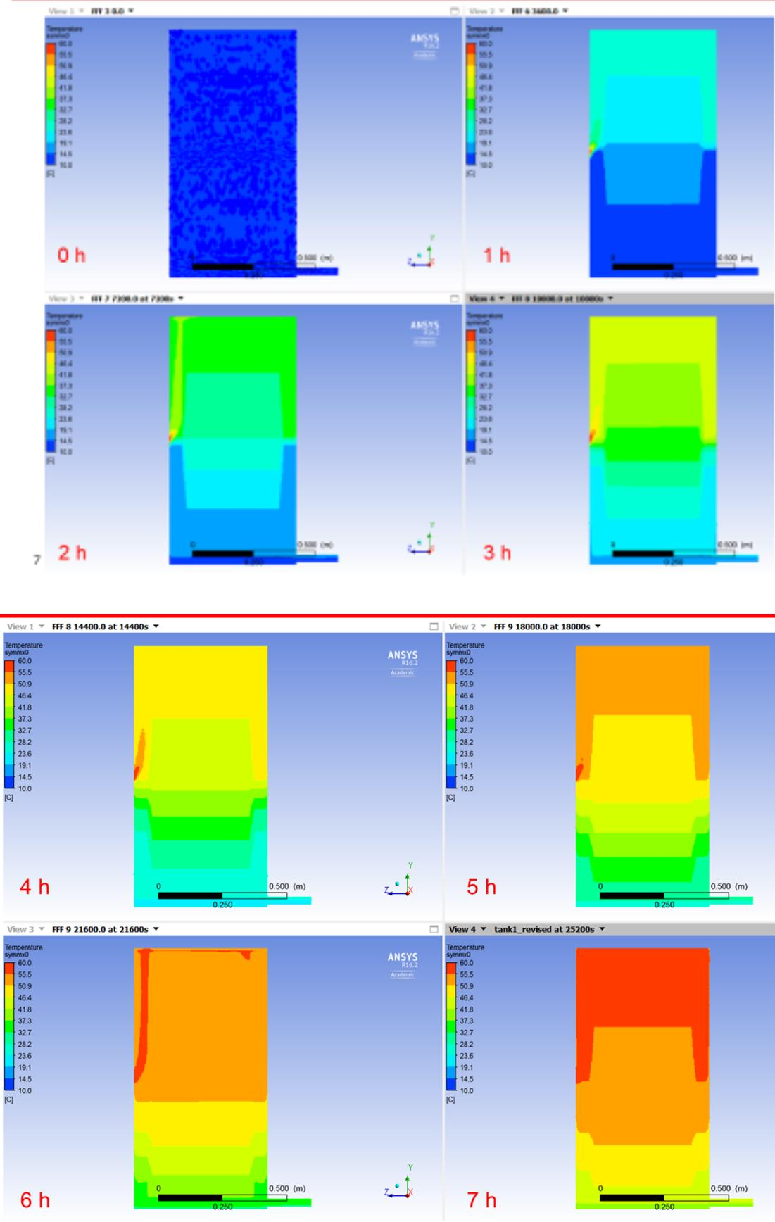
Figur 4. Heat storage temperatures during charge.
