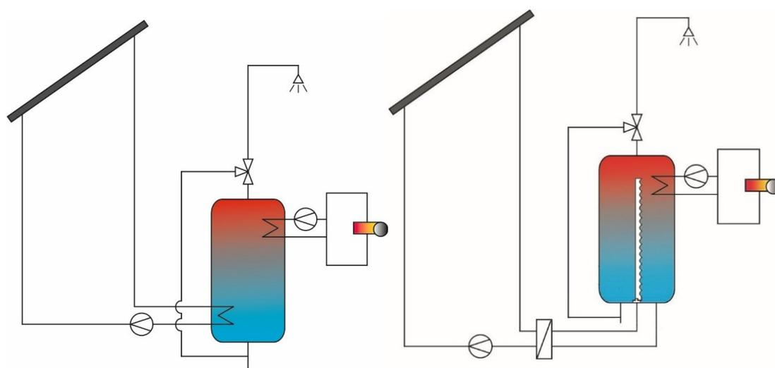
Figure 1. Schematically sketches of investigated solar heating systems.
