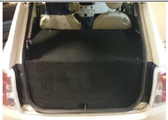
Figure 10 The cover of the technical room, which is placed at boot and back seats in the Fiat e500
