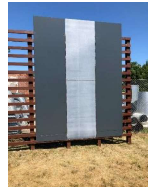
New BIPV technology from Danish Solar Energy, with light grey panels in the middle was demonstrated by Solarplan in combination with Rock panel facade, showing PV production quite near normal crystalline PV modules.
