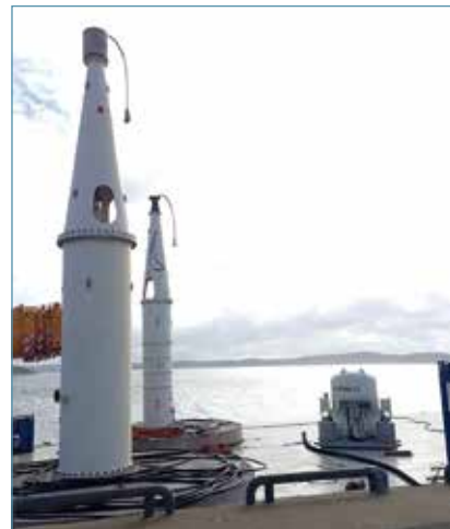
Picture from the Lysekil project. WECs to the left are deployed. Substation to the right will be deployed early 2015.
