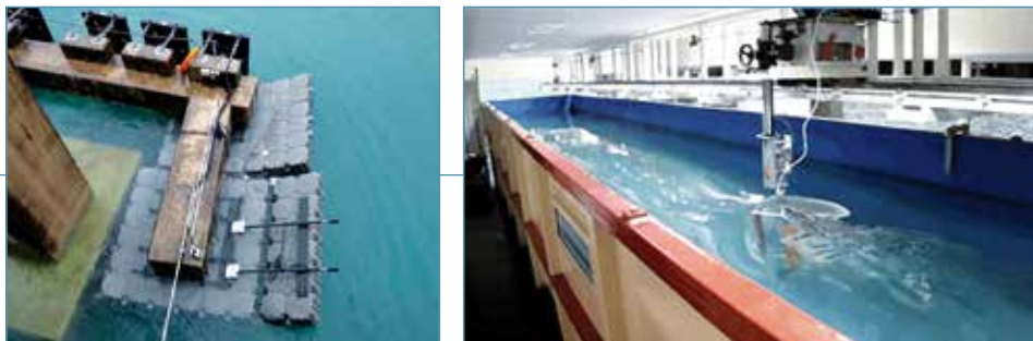
Floating hinged turbine support frame (Left) & Scaled (1:3) tidal turbine in tow tank (Right)
