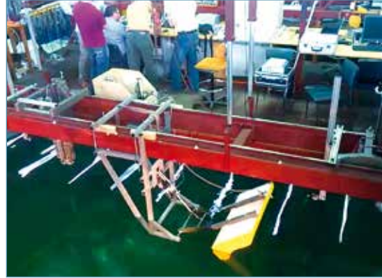
Wave tank test on 1:5 model scale of the Seapower system
