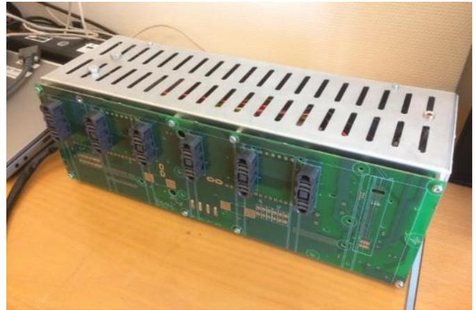
*3 The calibration and test system capable of calibrating six DCDC converters while mounted in the control-box*
