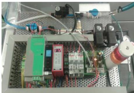
Figure 12 Fuel supply and fuel cell stack temperature control platform
