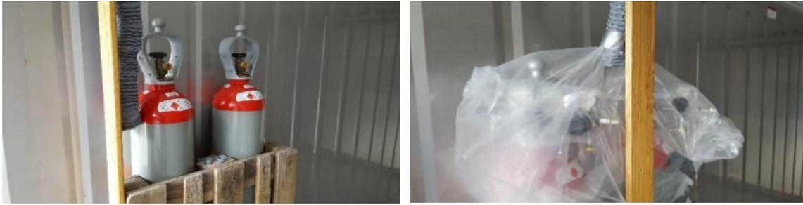
Figure 19 Regulators in  $-40^{\circ}\text{C}$  storage test
