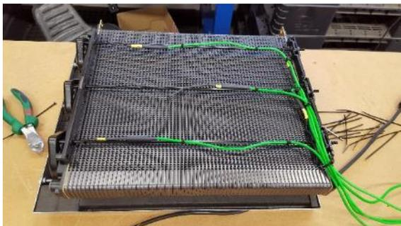
Figure 14a Fuel cell stack equipped with extra temperature sensors
