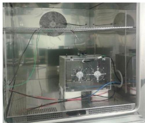
Figure 9 The fuel cell inside the climatic chamber
