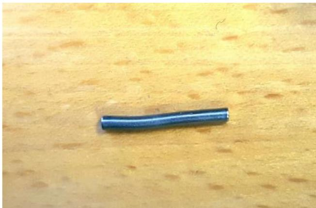
Figure 21 The needle that sits inside the regulator housing is bent.
