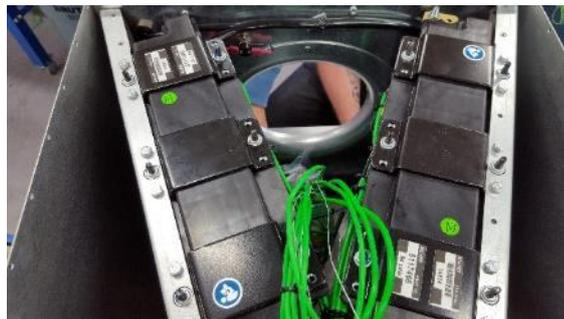
Figure 14b Fuel cell system with two stacks with extra temperature sensors.
