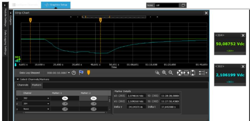
5 Measurement where the heating element is added and then removed again. The measurement changes 1.7%
