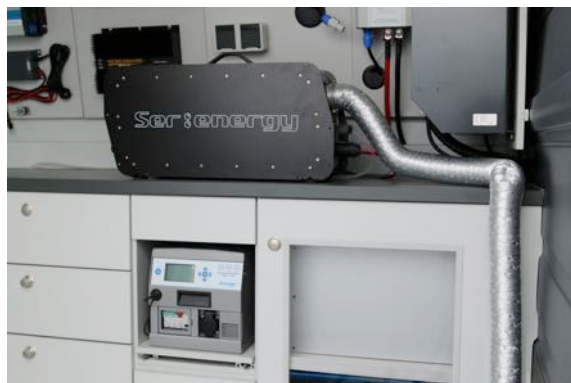
Figure 22 - Integration of a Auxiliary Hybrid Power system in LEAB Automotive's demonstration vehicle
