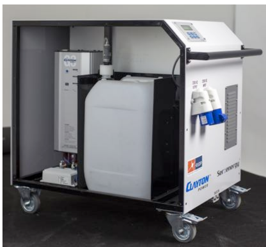
Figure 4 - Mobile APU - Fuel tank
