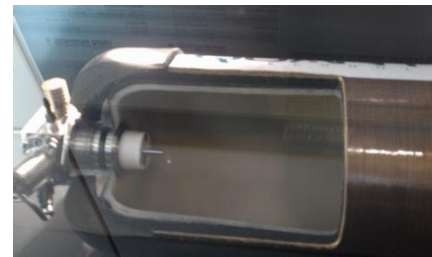
Figure 1 Quantum 700bar tank cut away
