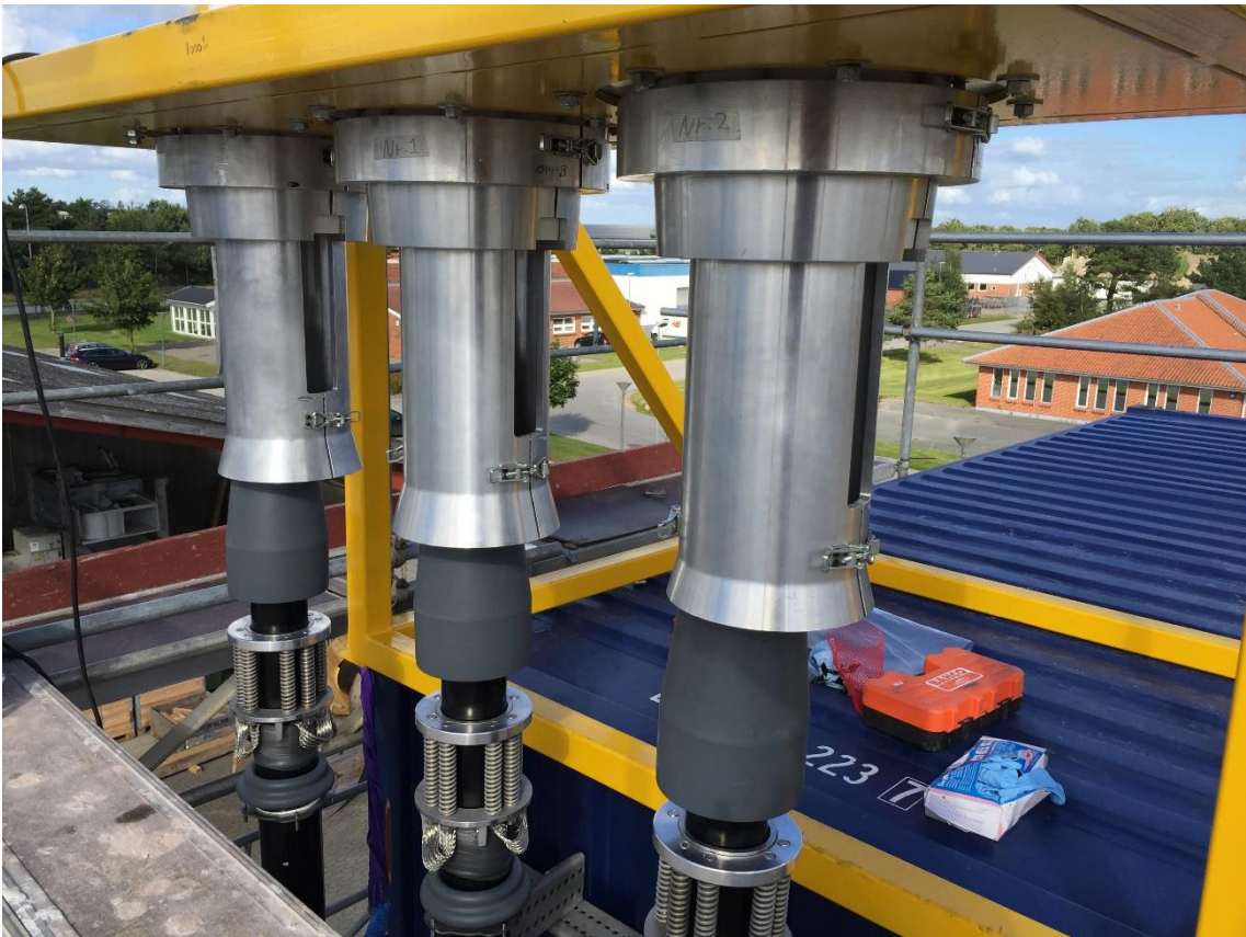
Figure 11 Cable connection with the HVAC Booster module.
