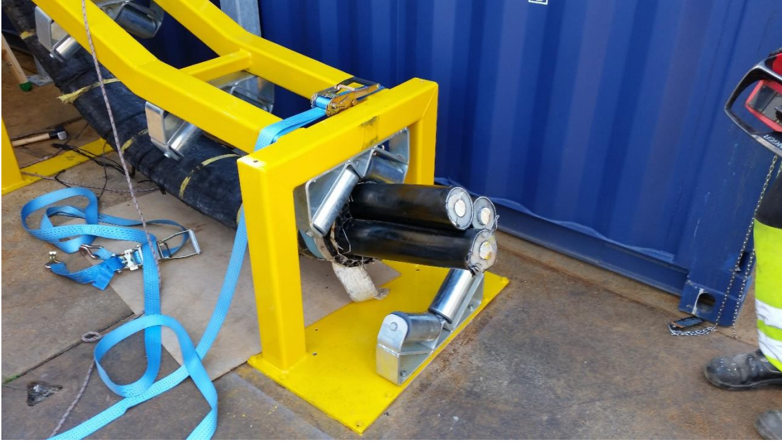
Figure 10 Cable entry in the bottom of the mock-up.
