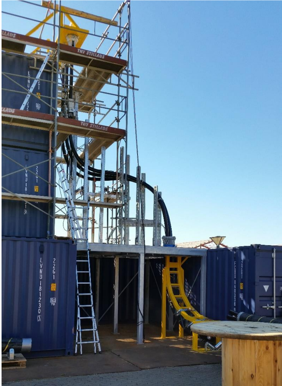
Figure 9 Full mock-up setup build from containers, scaffolds and Øglænd profiles.
