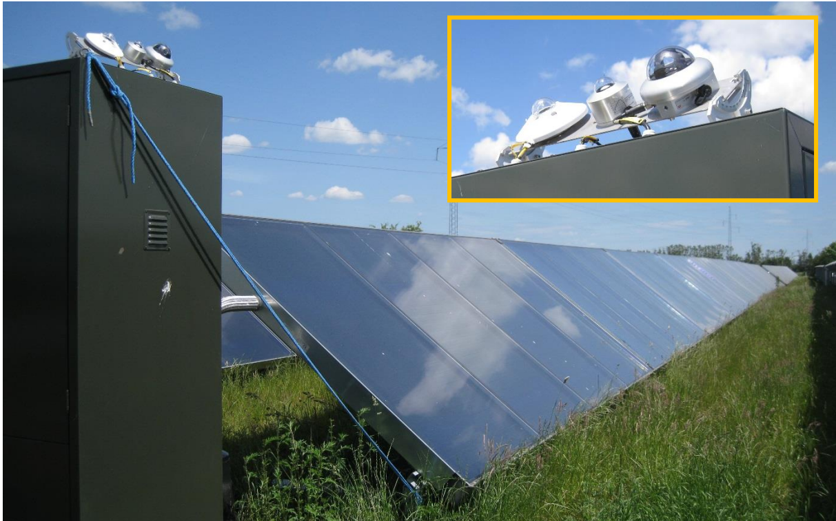
Figure 5.3.1. Solar radiation measuring from three different type of units. (From left to right: Kipp & Zonen SMP10, Indium Sensor type 3.3 and Delta-T Devices SPN1.)
