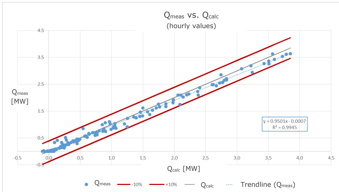
Figure 5.3.9. Hourly values of measured ( Q_{meas} ) and calculated ( Q_{calc} ) yield. The trendline for the measured values is seen as a dotted line. The linear expression for this line is seen in the blue box in the figure. The red lines indicates +/- 10 % of maximum calculated yield in the period.
