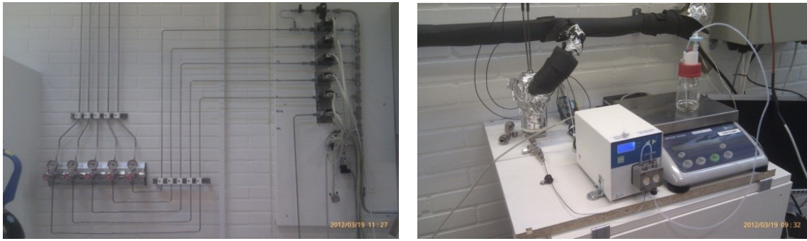
Figure 2: Gas supply system of CO, CO 2 , N 2 , N 2 and CH 4 (left) and toluene-solution pump (right)
