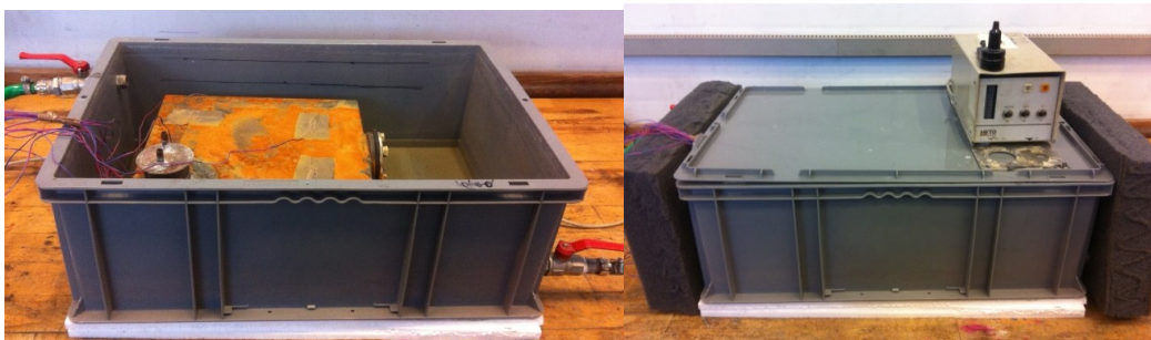
Figure 12. (a) Steel unit placed the thermostatic bath. (b) Closed thermostatic bath with controller.
