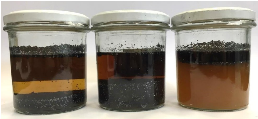
Figure 6. SAT samples with 1%, 2.5% and 5% CMC with graphite flakes on top after 14 days at 90°C.
