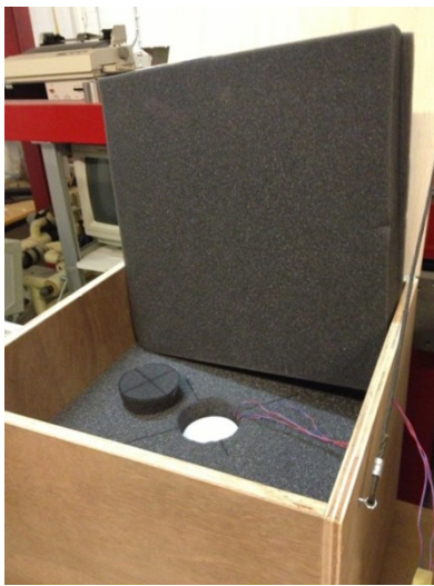
Figure 2. Well insulated box for heat content measurements by heat loss method.
