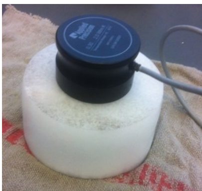
Figure 8. Applied Precision surface probe for measuring thermal conductivity of SAT sample.
