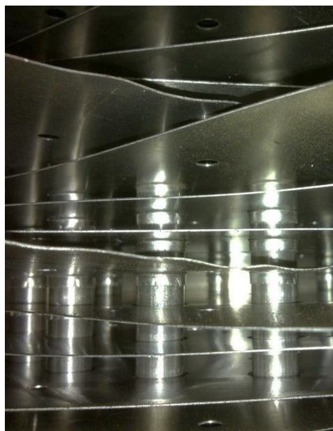
Figure 20. Internal heat exchanger of stainless steel pipes and aluminium fins.
