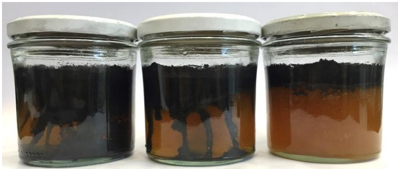
Figure 5. SAT samples with 0.25%, 0.5% and 1% Xanthan rubber with graphite powder on top after 14 days at 90°C.
