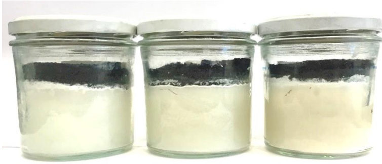
Figure 4. Three samples of SAT with thickening agent with a layer of graphite and SAT on top.
