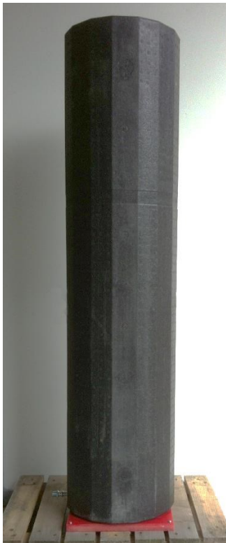
Figure 19. Cylindrical heat storage unit with insulation.
