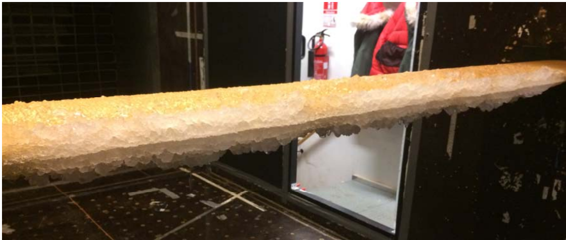
Figure 1: Glaze ice case at 4deg angle of attack
