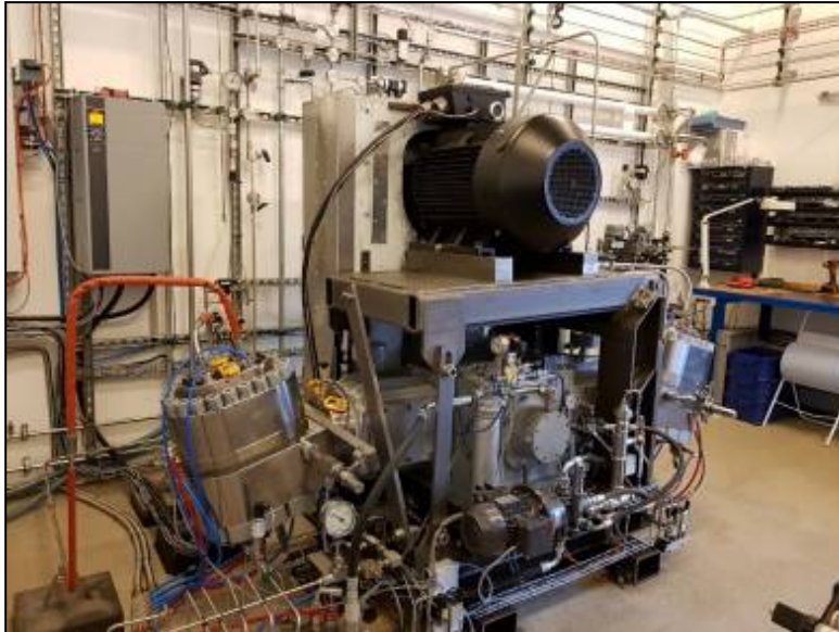
Figure 5.4.1.1 – Laboratory compressor prototype
