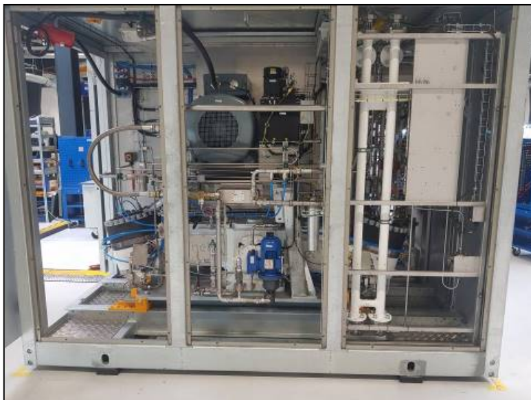
Figure 5.4.1.2 – Compressor prototype integrated into HRS
