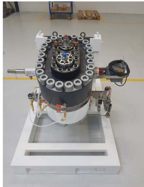
Fig. 5.2.1.1 1st stage compressor head
